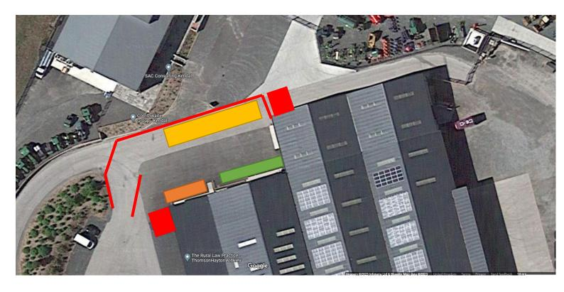
The x2 red squares represent where we will have additional lighting towers alomng with the external flood light already avaliable on the building, the lighting towers will be fenced off.
