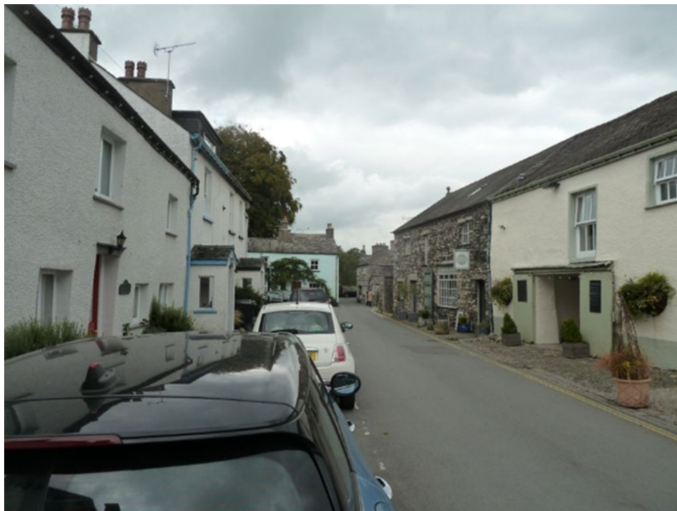
Figure 2 Cavendish Street in 2022. Removal of traditional render has a detrimental impact on character and appearance. Rubble surfaces were most likely never intended to be exposed.
